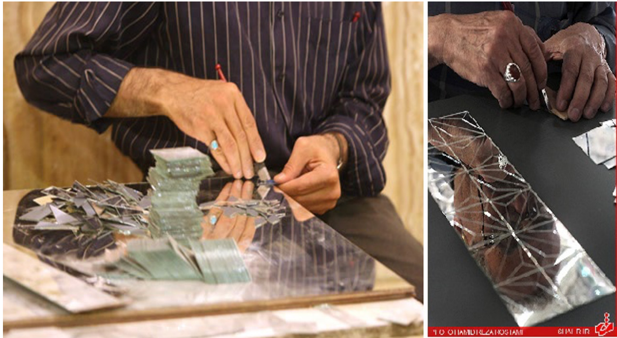
Figure 3: Creation of the Mirror-tiles from a full mirror plate. Source: RIBNews, Mohsen Rahimi Anbaran, www.tabnak.ir .
