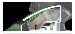
Figure 21. Section through dormitory unit. Note cyberspaces extending beyond lower living area and above vault of upper sleeping loft. Looped railing supports a mobile laser projector that may shine on scrim or on ceiling vault.
