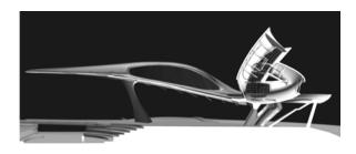
Figure 23. Section through Observatory and tensile cloud structure. Note optical assembly in fly structure of Observatory.
