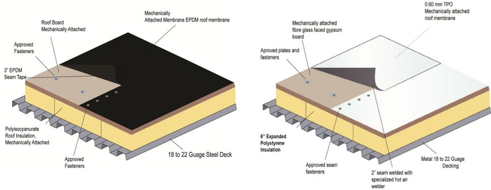
**Fig. 2.** Comparison between existing assembly (left) and proposed retrofit (right) (courtesy of Platinum Roofing, Inc.)
