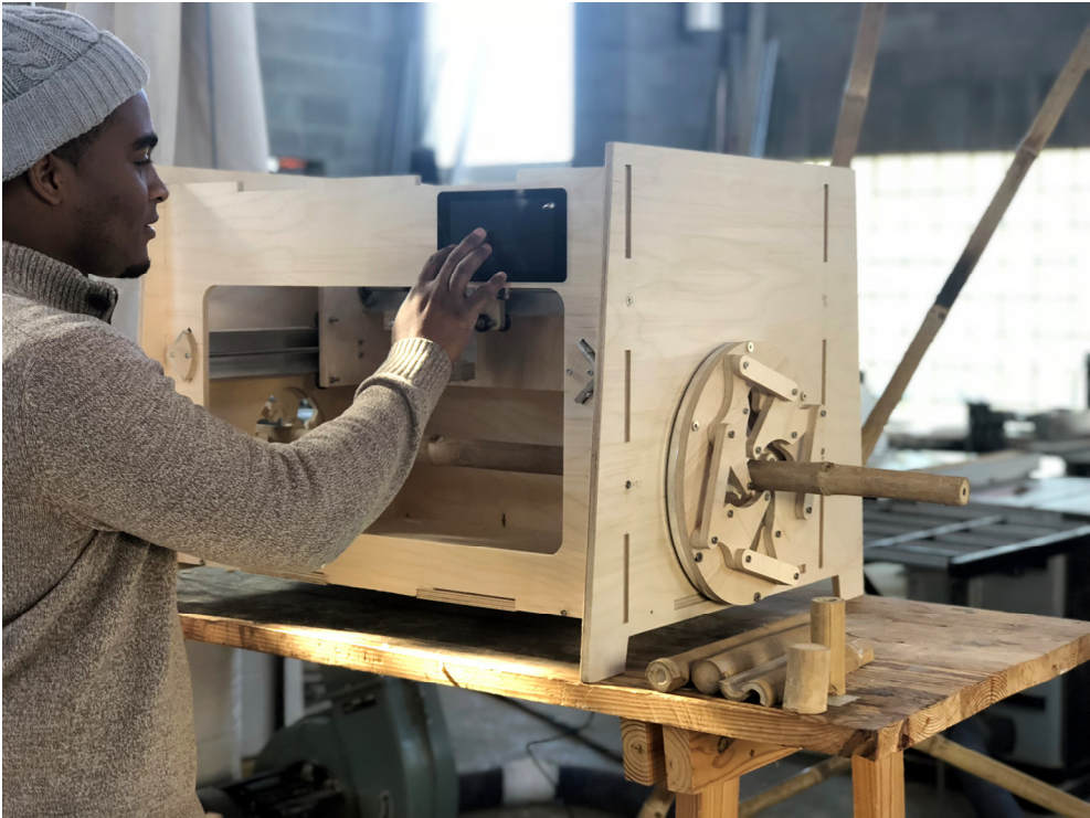
Figure 7: Integrated scanning, parametric part selection, and CNC routing machine for bamboo pole construction. Source: (Author 2019)
